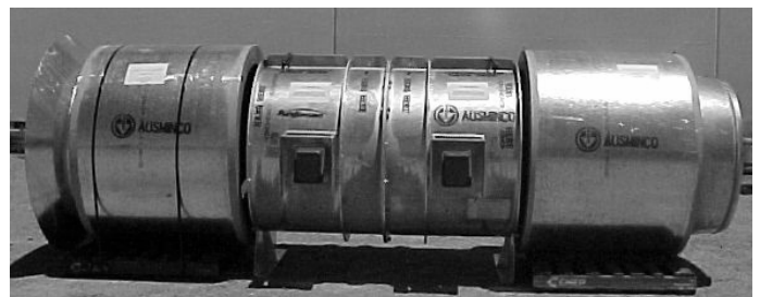
Figure 2. Typical metalliferous (hardrock) mine auxiliary fan
