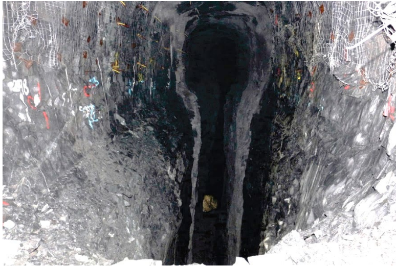
Figure 14. Improvements made to the narrow vein stope at Eleonore mine in Quebec. Note the reduction in stope damage with hanging wall intact. The fragmentation specification of muck < 400 mm (16 in) was also met. Dilution was drastically reduced to less than the original specification of 10%.
