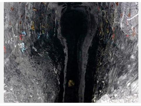
After: This photograph shows the narrow ore vein almost completely recovered with little dilution and virtually no damage owing to a blasting pattern that was redesigned and expanding using the AEGIS Break Analyzer software.
