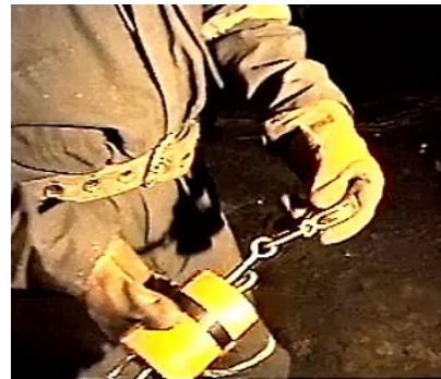
Frame 2 - The completed hardwood wedge assembly ready to be inserted into boreholes.
