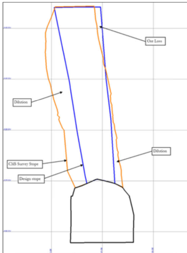
FIG 6 - Section showing Dilution and Ore Loss
