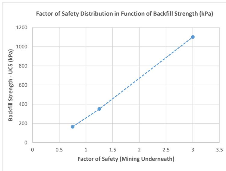
Figure 5: Evolution of the Safety Factor Associated with Backfill Sill Exposure in Function of Backfill Strength (kPa)
