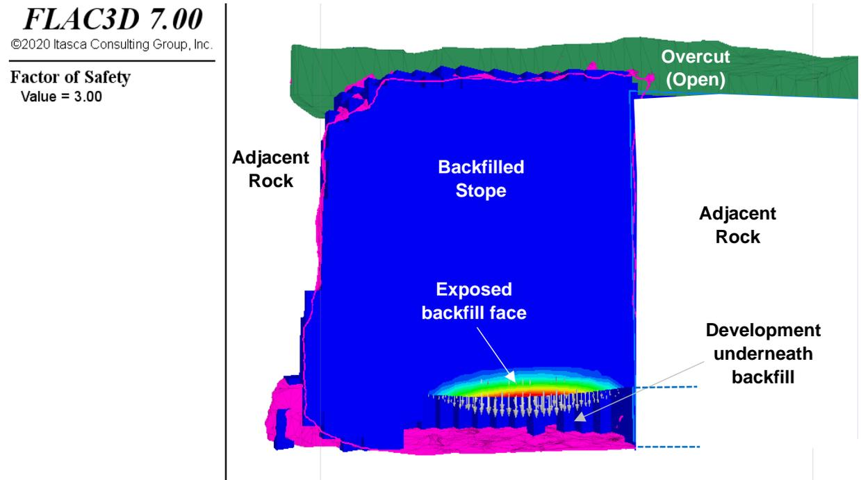
Figure 4: Displacement Magnitude Isocontours and Velocity Vectors showing the area of potential Instability of the Backfill and the corresponding deformed mesh (Exaggerated x 1.3)
