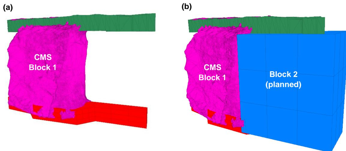
Figure 1: (a) Isometric view showing the geometry of the mining area consisting of top and bottom drifts and a mined-out stope. (b) Planned Block and Exposure of the End wall of the CMS
