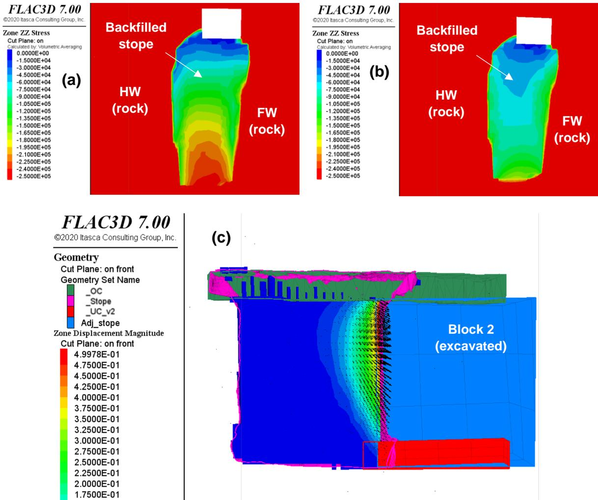
Figure 2: Isocontours of the vertical stresses ( $S_{zz}$ ) on cross section view at mid-strike length of (a) backfill 1 (low strength); (b) backfill 2 (medium strength) and (c) the Unstable section of backfill with displacement contours and vectors (long section at mid-width)
