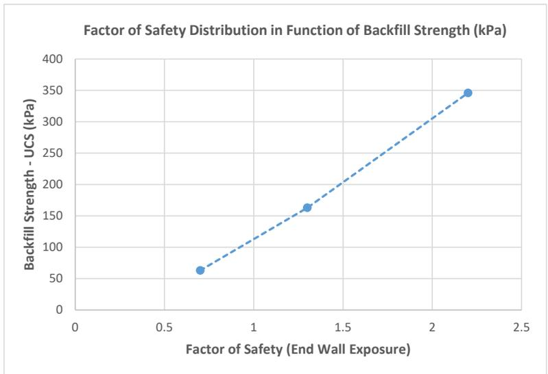
Figure 3: Evolution of the safety factor associated with the end wall backfill exposure in function of backfill strength (kPa)
